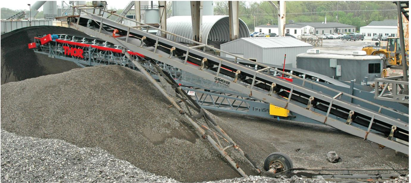
**After separating, the fine material goes to the new automated telestacking conveyor then to a covered storage building.**
